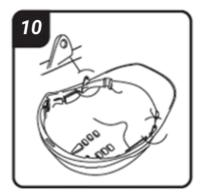
1. The chin strap is an accessory that must be fitted into the holes in the hull (fig. 10)
